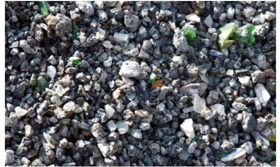
Hydro-cleaned granulate: free from sludge and extraneous material
